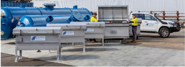
Como Engineers are suppliers of heavy duty 304 Stainless steel, rubber lined electrowinning cells. Proven, standard designs which are available in a range of cathode sizes.
