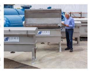
The cells in these images are destined for mines in Western Australia and Mali (600mm x 600mm models shown with non-drip lid design and spring hinges for easy opening and closing).
